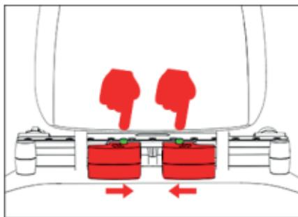
3. Remove the two side supports. Slide out the sliding rod.
